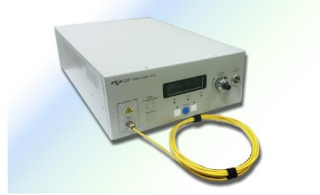
All-fiber design and splicing technology make the laser more compact compared to traditional rod or disc DPSS lasers. The peak intensity of a laser pulse with a duration of only a few picoseconds is so high that nonlinear/multi-photon absorption occurs, resulting in a very precise "cold" process with little thermal effect.
