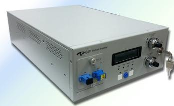
The AMP-EFA-FS-HP-U does not need water cooling or replacement parts, only 110/220V AC power supply is needed to obtain high energy and high peak power pulsed laser.
